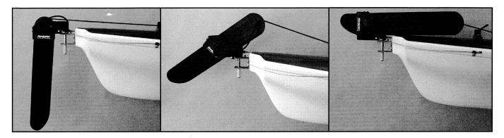
Instead of pivoting 270° to stow itself on deck, the Navigator rudder slides through a pivoting sleeve.
